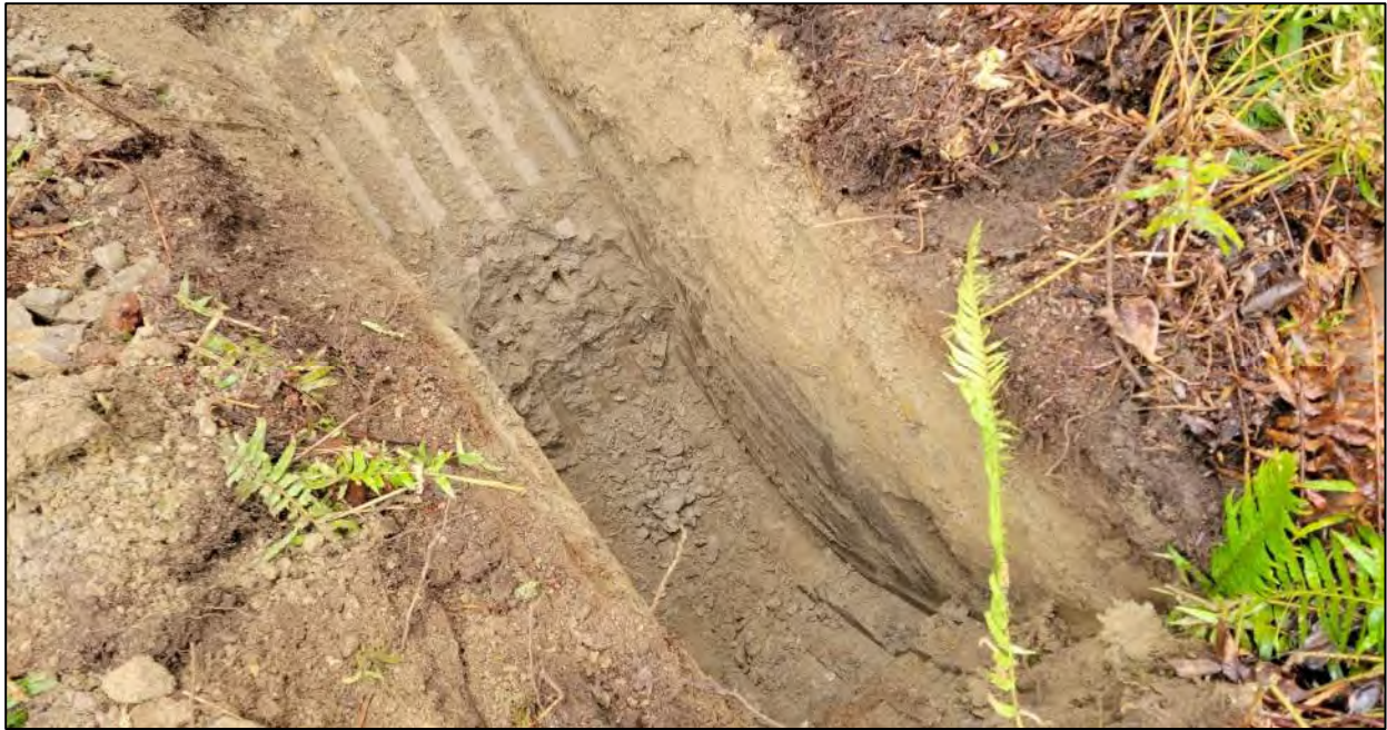
Image 4. View of excavation at TP-3 exhibiting typical Upper Glaciomarine Drift deposits.
